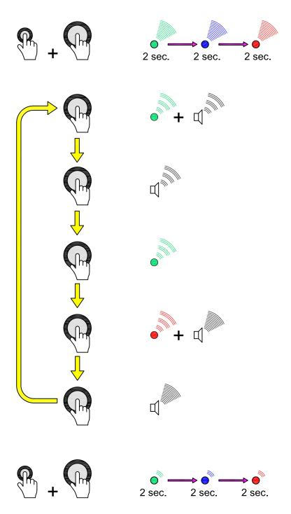
Turn on: Press the **small button first**, and then holding the small button press the big button. In 6 seconds the device goes into operation mode.
